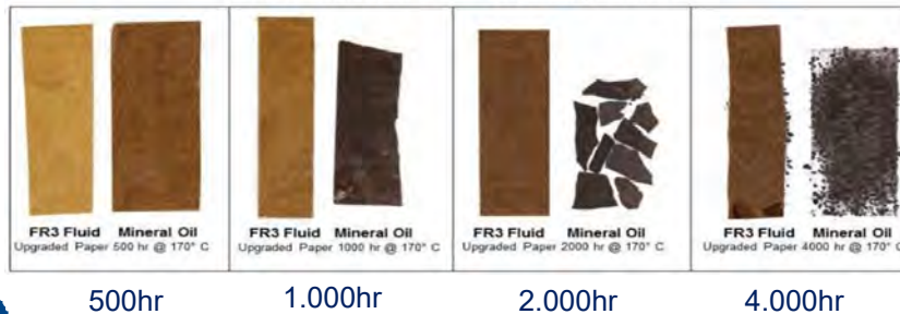
FR3™ natural ester fluid vs. Mineral oil Sealed Tube Test - IEEE C57.100, Annex B
